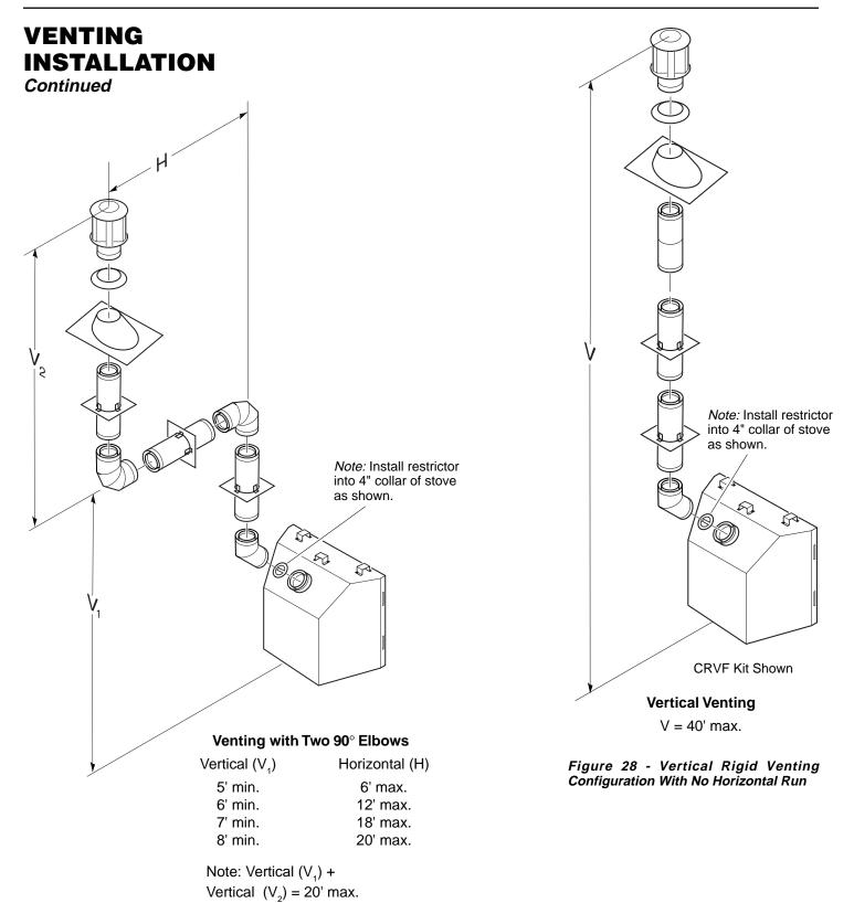
Figure 27 - Vertical Rigid Venting Configuration Using Two 90° Elbows
